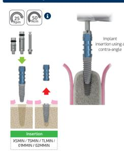
Insert the implant into the surgical site, controlling both the direction and angle of the implant. When inserting the implant with a contra-angle, use a maximum speed of 25 rpm. The recommended insertion torque ranges from 35 to 50 Ncm, according to each case, and is not limited to a single torque.
